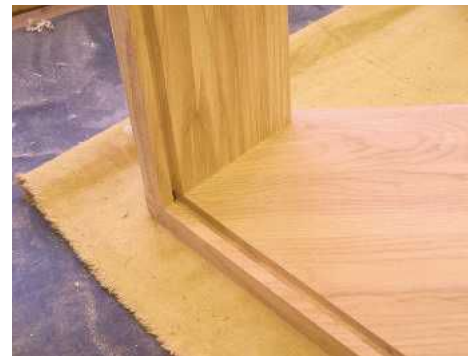
▲ Pic.8 Form grooves for the side panels in the front uprights and the top and panel. They should line up on assembly
